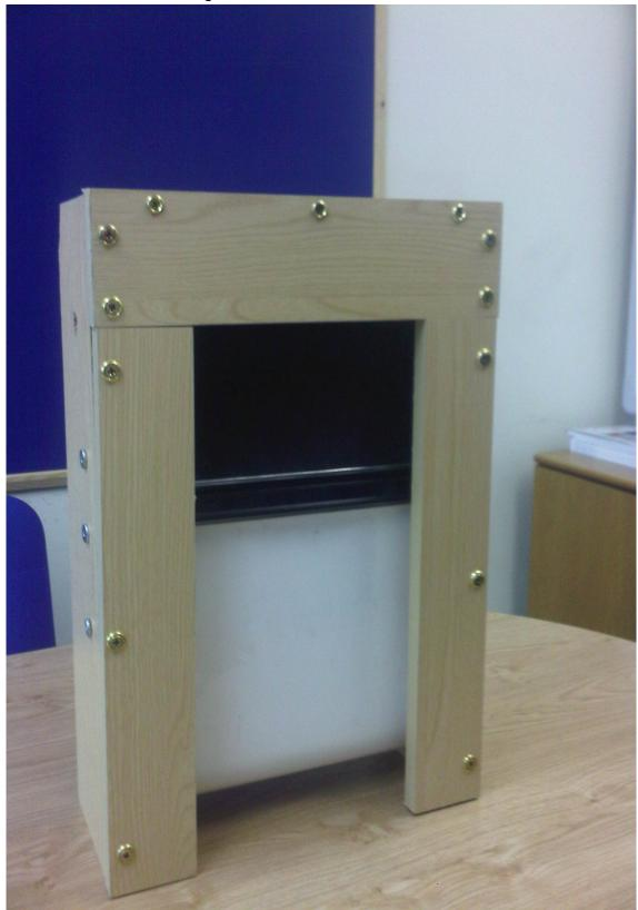
Stage 1 Remove facing from front of rollerboard using a Phillips head screw driver.
