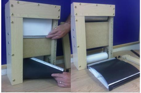
Roll the entire new surface into a tube, with the writing surface inside the tube, and place at the bottom of the board behind the facing.
