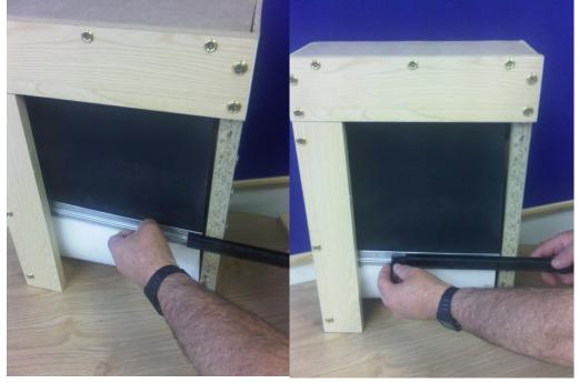
Before the black plastic closer is pushed fully onto the blade, press on the end cap on the far side (the leading end when pushing on) then fully push on the blades pressing the end cap on when it is against the far side leg. Add the other end cap to the open end.
